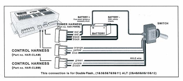
IV. Wiring Control Harness. Combination of different wires (ORANGE, YELLOW, BLUE, PURPLE, and BROWN) allow for different flash patterns; (see table). The GREEN wire from Power Harness enables High/Low Power function; (when off, it's at High Power, and when on, it's at Low Power. The remaining unused wires may be removed or left in place for future alterations.
