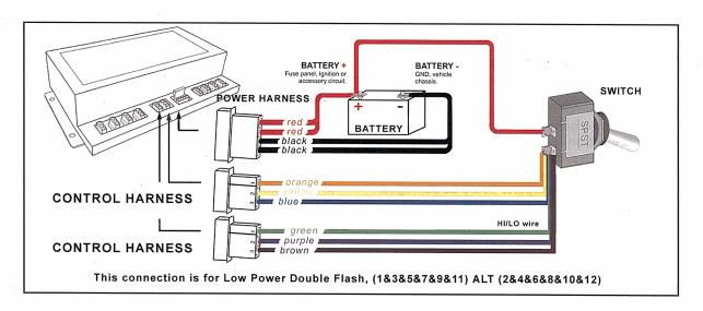
IV. Wiring Control Harness. Combination of different wires (ORANGE, YELLOW, PURPLE, and BROWN) allow for different flash patterns; (see table). The GREEN wire from Power Harness enables High/Low Power function; (when off, it's at High Power, and when on, it's at Low Power. The BLUE wire is reserved for future function. The remaining unused wires may be removed or left in place for future alterations.
